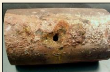
Oxygen Pitting in a Standby Boiler
