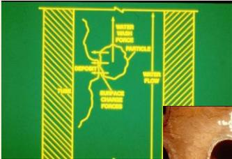
Once scale has formed on a metal surface, this deposit will attract other charged particles in the boiler water.
