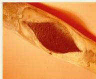
Water Tube Boiler deposits build up in the tubes causing thin or thick lip bursts. As the metal of the tube over heats, the tube bulges, then bursts. High temperature stress cracking, the tube over heats, becomes hardened steel which is brittle and cracks
