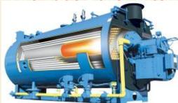
The internal design of a fire tube boiler starts with the combustion in the center fire tube or Morrison tube.
