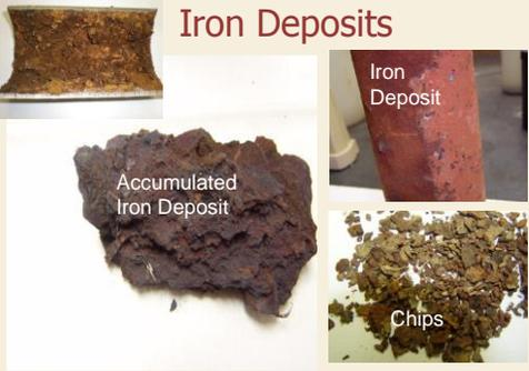
The slide features four photographs illustrating iron deposits. Top left: A brown, crusty deposit on a surface. Middle left: A dark, irregular flake labeled 'Accumulated Iron Deposit'. Top right: A red pipe with a dark coating labeled 'Iron Deposit'. Bottom right: A pile of greenish-brown particles labeled 'Chips'.
