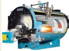
Wet Back boilers redirect the heat of combustion off of a wetted section picking up more heat at the end of the first pass and can take more over heating.
