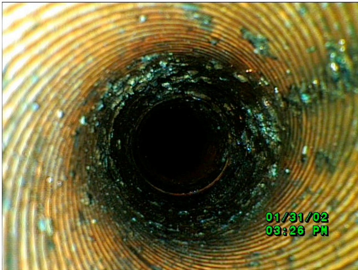
Source: Hoffman & Feige Metallurgists Fiberoptic Scoping reveals severe deposition and corrosion.
